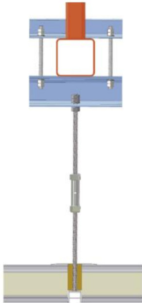
Fig. 13a - Fastening of ceiling panel with insert
