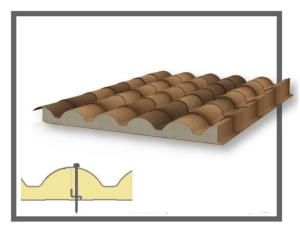
These types of panels are made up of a pre-lacquered steel sheet on the upper part and a thin layer of embossed aluminum on the lower part, between them a core of rigid foam injected between the two sheets in a continuous manufacturing process (PUR).
