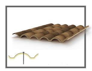
These types of panels are made up of a pre-lacquered steel sheet on the upper part and a thin layer of embossed aluminum on the lower part, between them a core of rigid foam injected between the two sheets in a continuous manufacturing process (PUR).
